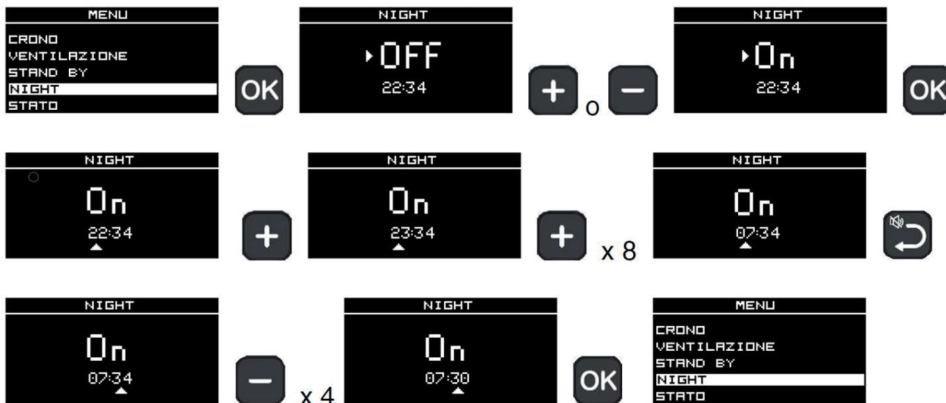
The switch ON time is shown on the main display.
