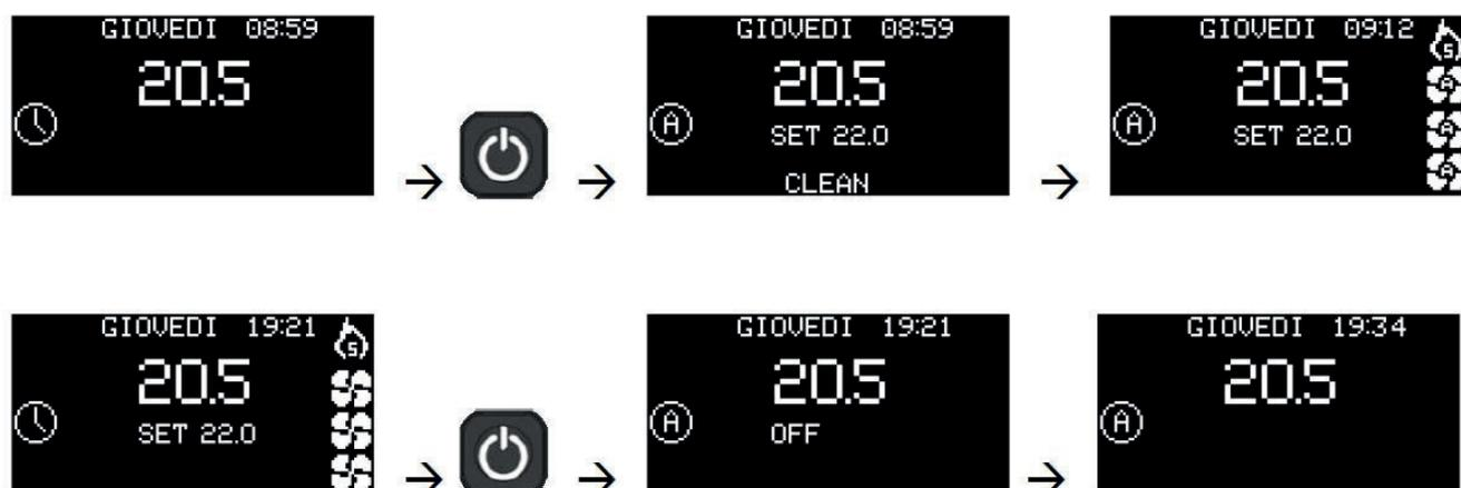
The switching on and off force the move from Crono to Automatic mode with the pre-set Set Room and Ventilation.
