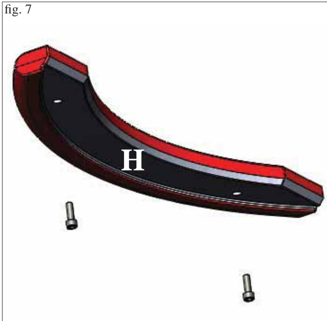
Fig. 7 Lightly tighten the 2 milled M4 pins provided on the back of the upper ceramic element (H).
