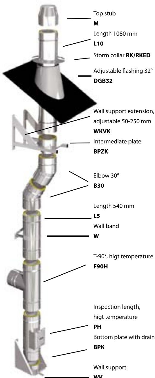
Between two elements the connection is established by a locking band. At least every 4m the chimney is to be secured by a wall band. The free length above the last wall band may not exceed 3 m. Otherwise a steel rope or a steel construction are necessary for stability.
