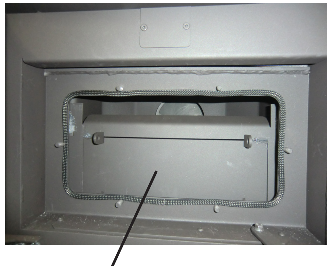
Fig. 5 Separating wall water-heat exchanger
