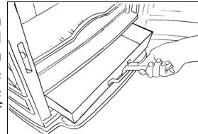
Relatively speaking, burning wood produces little ash and it will not be necessary to remove it each time daily. Moreover, wood burns better on a bed of ash.
