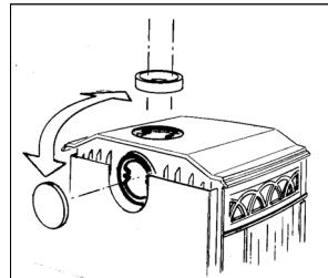
Remount the removed heat shield, if any, before connecting the appliance to the chimney.
